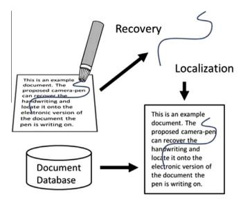
Fig. 1. Processes required for camera-pens.
