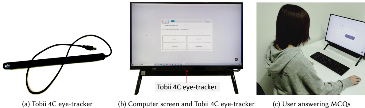
Fig. 6. Data recording proceedings for confidence estimation, (a) eye-tracker used, (b) computer screen with an example question and eye-tracker fixed at the bottom, and (c) eye-tracker recording user’s eye-gaze while answering MCQs.
