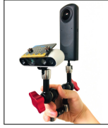
(a) Omnidirectional camera (810 g)
