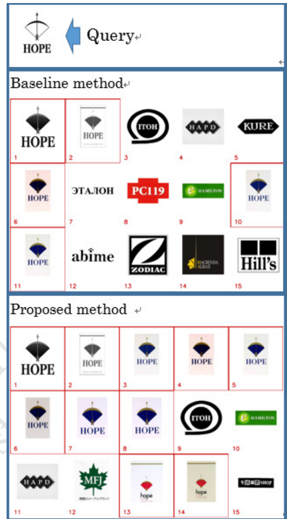
Figure 11: An example in which the accuracy was improved by feeding back a relevant image to the query image. The upper row shows the query image, the middle row shows the retrieval result of the baseline method and the lower row shows the retrieval result of the proposed method ( N = 1 ). An image surrounded by a red rectangle is the relevant image.
