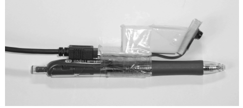
Figure 3 The camera pen. It contains an ordinary ballpoint pen and a tiny USB camera.
